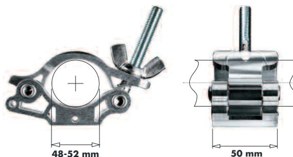
**LP EYE COUPLER:** industry standard Ø48-52mm pipe clamp range, load capacity up to 500kg, TUV certified. Available with a full range of fittings, including M12 bolt with nut, 28mm TV spigot, lifting ring.
