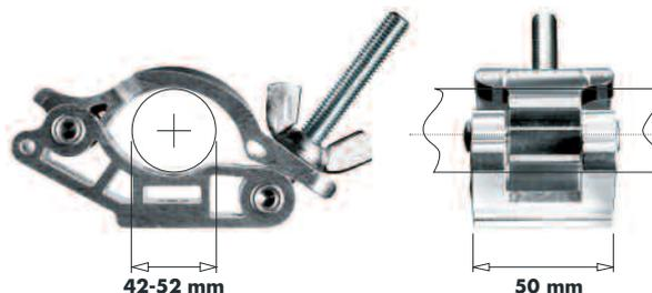
**MP EYE COUPLER:** wider Ø42-52mm pipe clamp range, special flattened jaw design for easier fixing in tight spaces, load capacity up to 500kg, TUV certified. Available with a full range of fittings.
