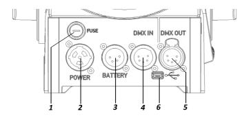
1 Fuse holder 2 AC power in 3 Connector for battery pack 4 DMX input 5 DMX output 6 USB connector
